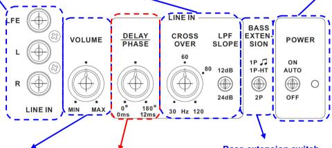
**Volume level setting** is determined by the efficiency of front speakers. It is not an indication of whether the sub can play louder or not.
