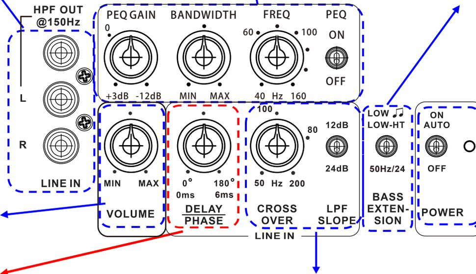
Volume level setting is determined by the efficiency of front speakers. It is not an indication of whether the sub can play louder or not.
